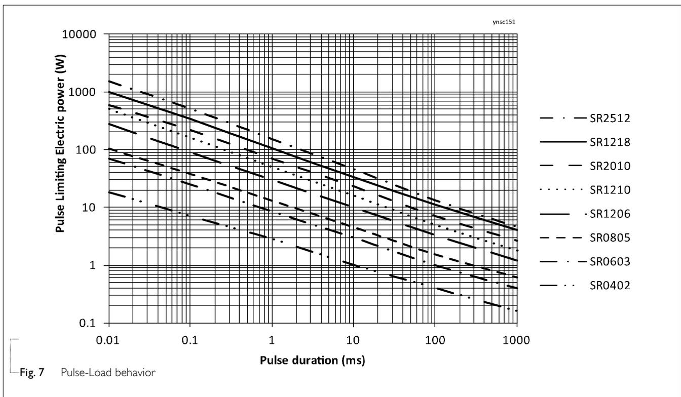
Fig. 7 Pulse-Load behavior
