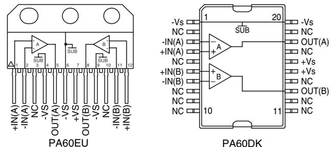
FIGURE 3. External connections
