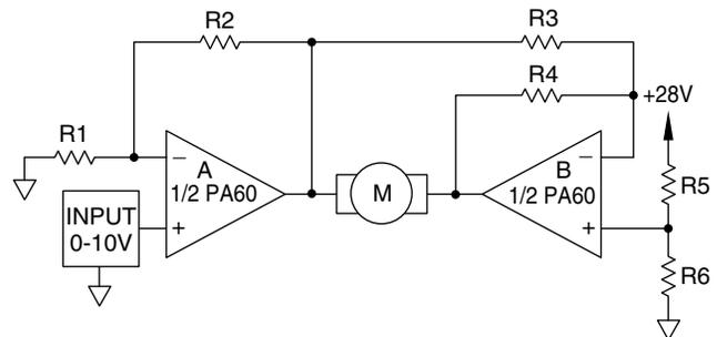
FIGURE 2. Bi-directional speed control from a single supply
