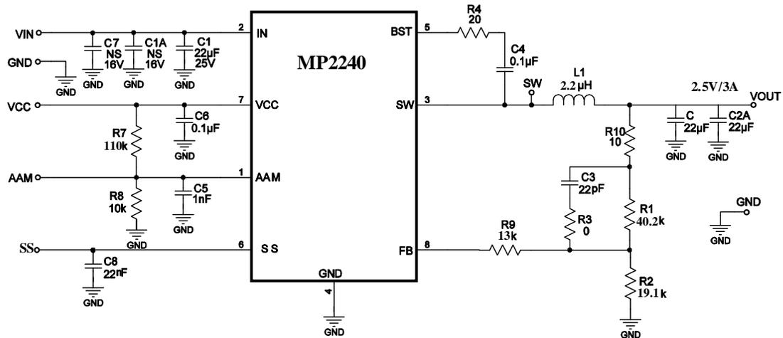
**Figure 10: 12V<sub>IN</sub>, 2.5V/3A Output**
