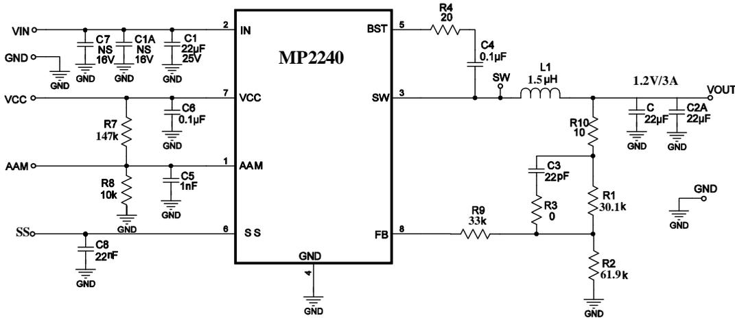
**Figure 8: 12V<sub>IN</sub>, 1.2V/3A Output**
