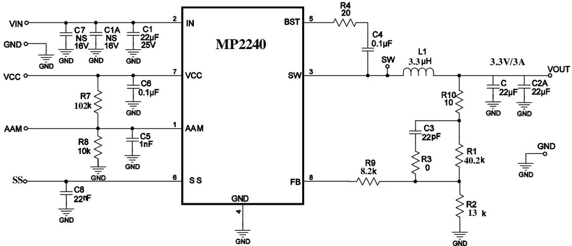
**Figure 11: 12V<sub>IN</sub>, 3.3V/3A Output**
