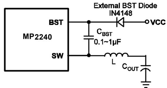
**Figure 6: Optional External Bootstrap Diode to Enhance Efficiency**
