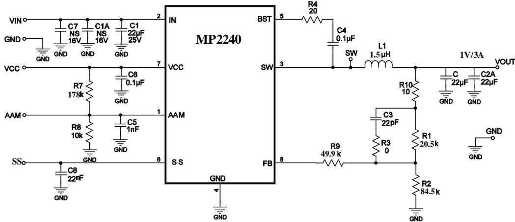
**Figure 7: 12V<sub>IN</sub>, 1V/3A Output**
