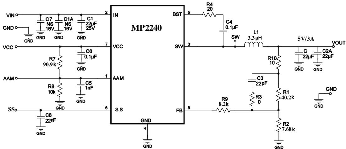
**Figure 12: 12V<sub>IN</sub>, 5V/3A Output**
