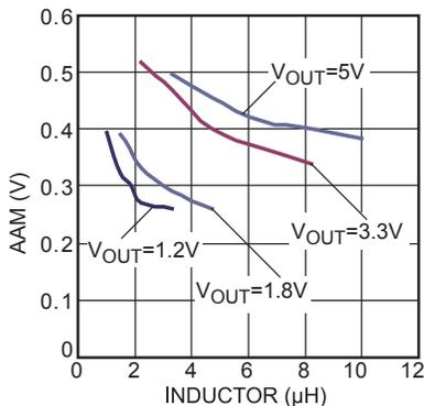
**Figure 5: AAM Values for Common Output Voltages (V<sub>IN</sub> = 6V to 16V)**
