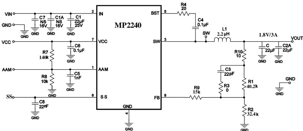
**Figure 9: 12V<sub>IN</sub>, 1.8V/3A Output**
