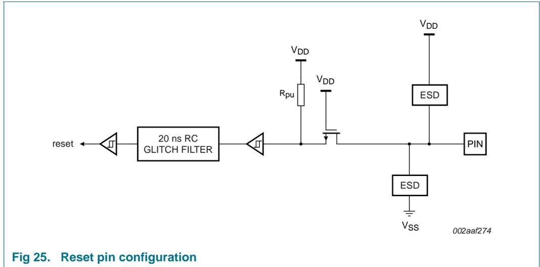
Fig 25. Reset pin configuration
