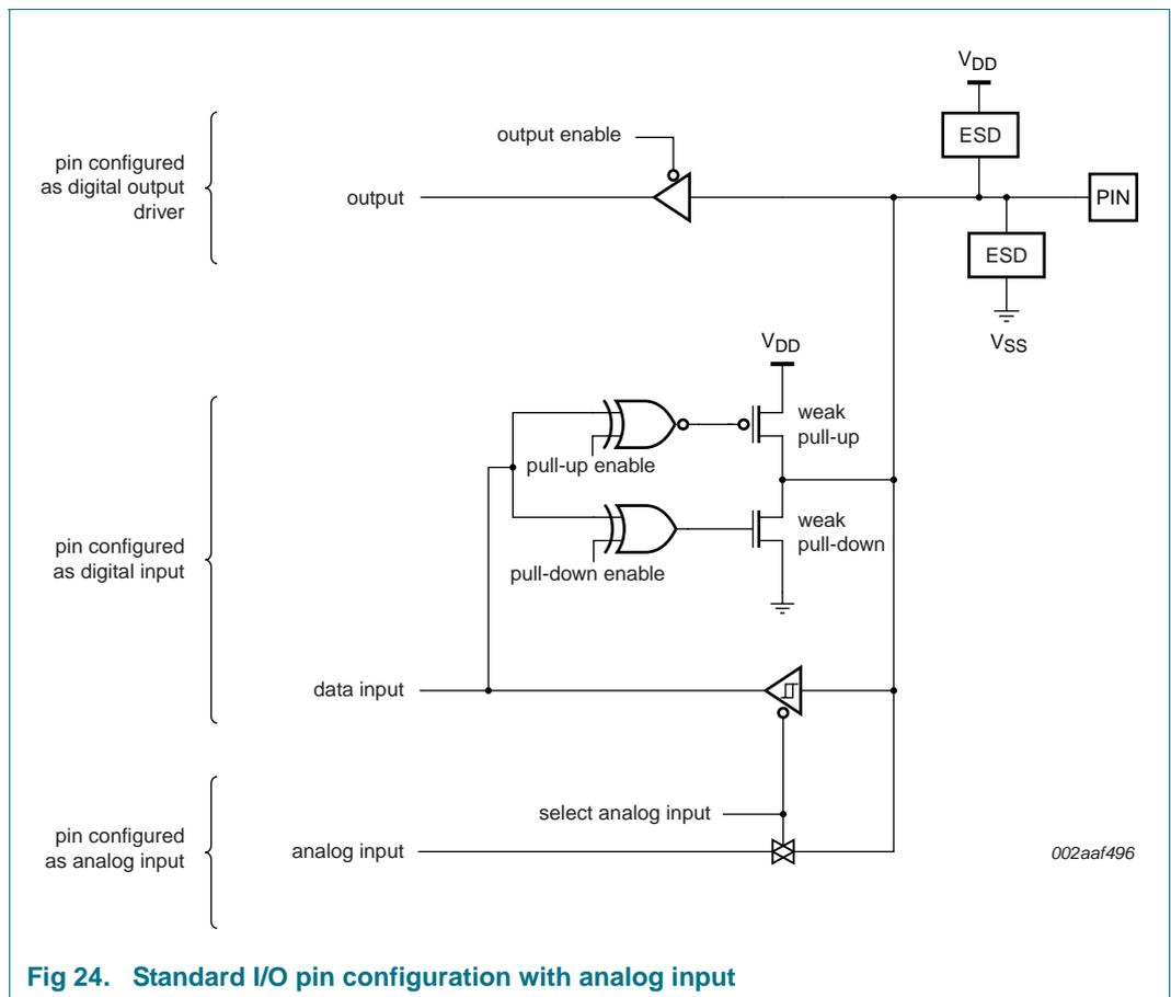
Fig 24. Standard I/O pin configuration with analog input
