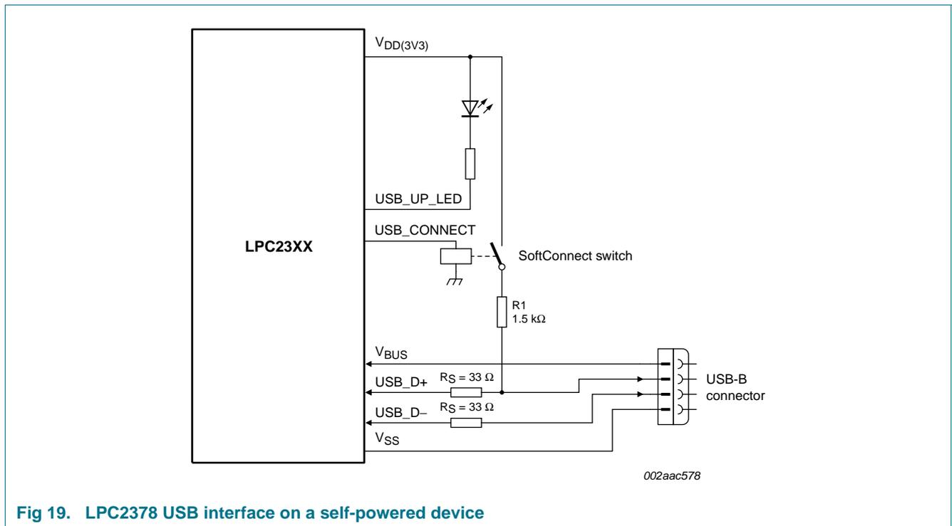
**Fig 19. LPC2378 USB interface on a self-powered device**
