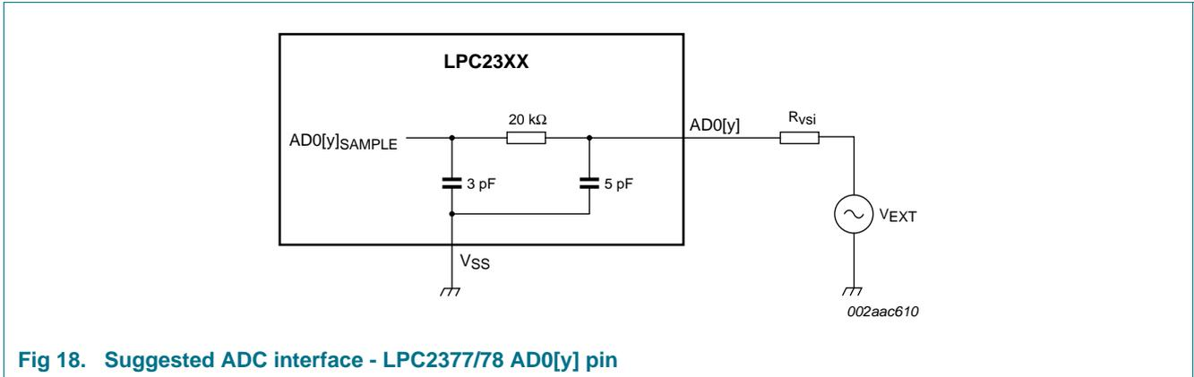
Fig 18. Suggested ADC interface - LPC2377/78 AD0[y] pin
