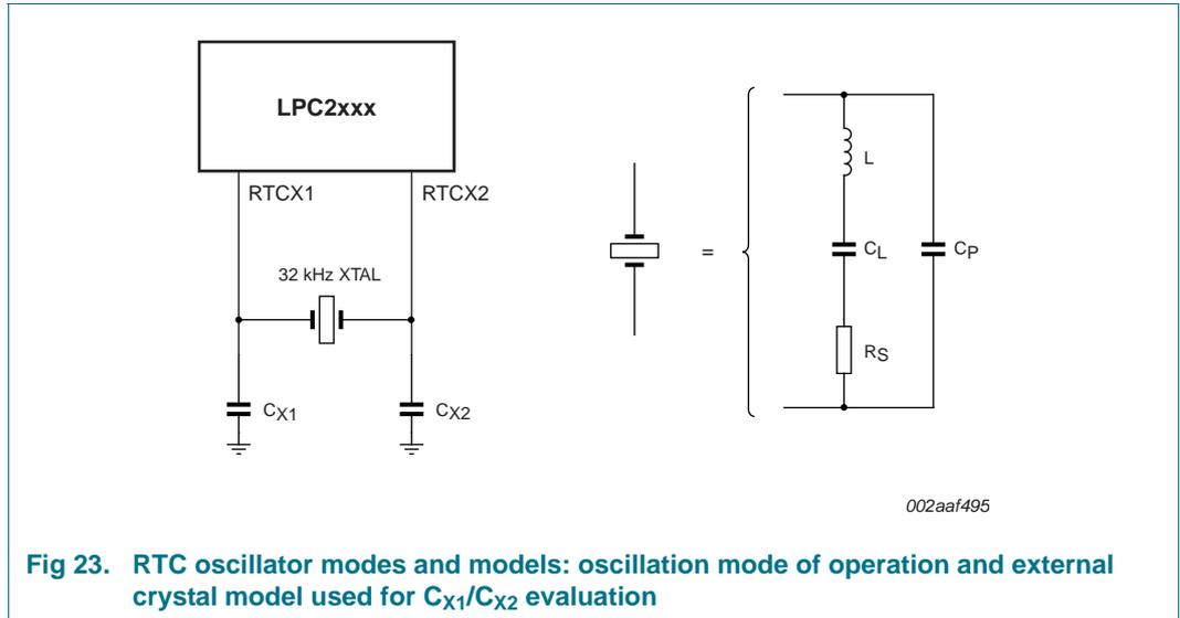
The RTC external oscillator circuit is shown in [Figure 23](#). Since the feedback resistance is integrated on chip, only a crystal, the capacitances  $C_{X1}$  and  $C_{X2}$  need to be connected externally to the microcontroller.
