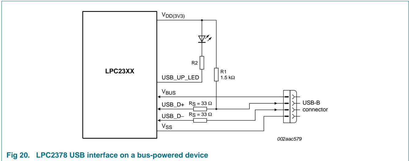
Fig 20. LPC2378 USB interface on a bus-powered device
