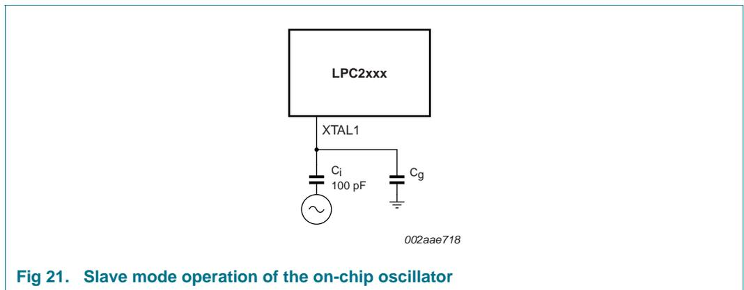
Fig 21. Slave mode operation of the on-chip oscillator
