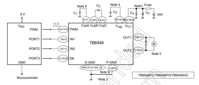
TB6549FG: Pins 1, 5, 6, 9, 13, 15, 16, and 19 are not connected. TB6549HQ: Pins 4, 5, 7, 8, 9, 13, 17, 18, 19, 21, and 22 are not connected.
