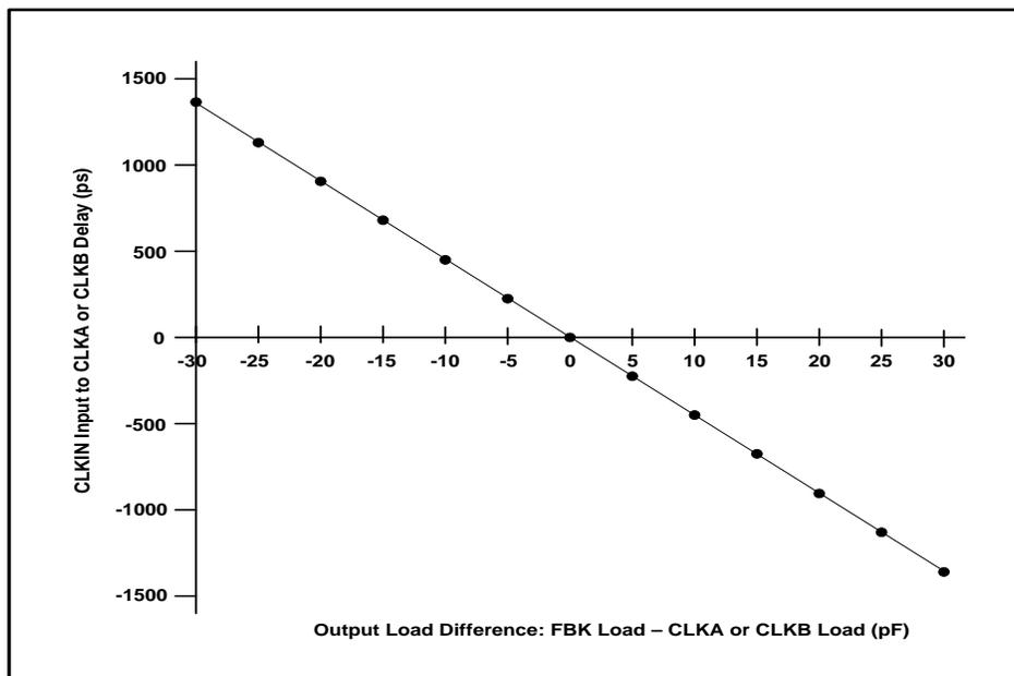
Figure 1. CLKIN Input to CLK A and B Delay
