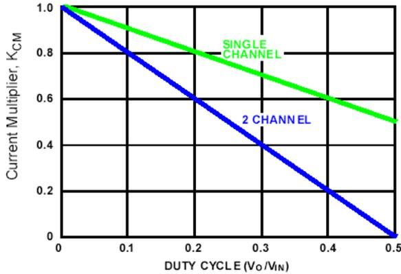
FIGURE 12. OUTPUT RIPPLE CURRENT MULTIPLIER vs DUTY CYCLE
