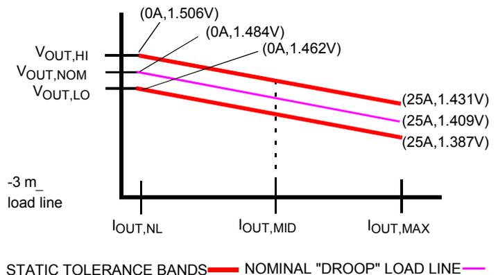
FIGURE 11. IMVP-IV ACTIVE MODE STATIC LOAD LINE
