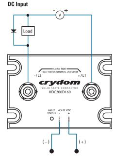
(E) Inductive loads must be diode supressed as indicated.
