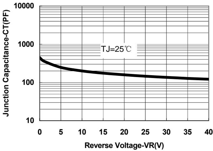
Fig.1-Typical Junction Capacitance
